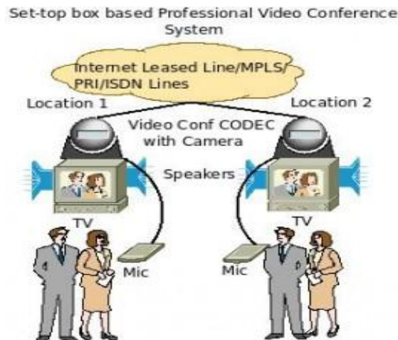
Fig. 3: Block diagram and Architecture of Professional Video Conference system
